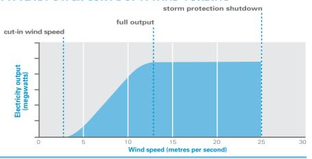
or a strong gale). At this point the turbine will automatically shut down to prevent damage.
